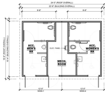
**\*Note:** This floor plan is comprised of two (2) mods and compliant for California.
